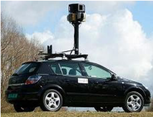
Figure 8. An example of a camera system mounted on a car. It is designed to cover a wide viewing range.
