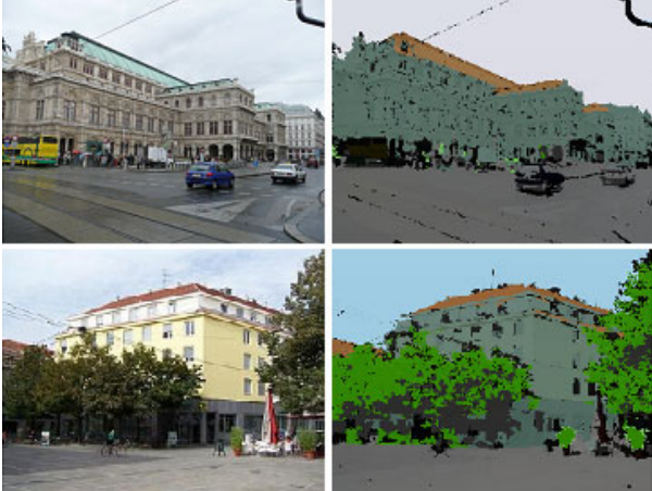
Figure 3. Original images (left) and semantic segmentation (right) [10]. Each class is represented by a color: building (dark green), sky (blue), roof (brown), vegetation (green), ground (grey), clouds (white). Black areas are considered unidentified.
