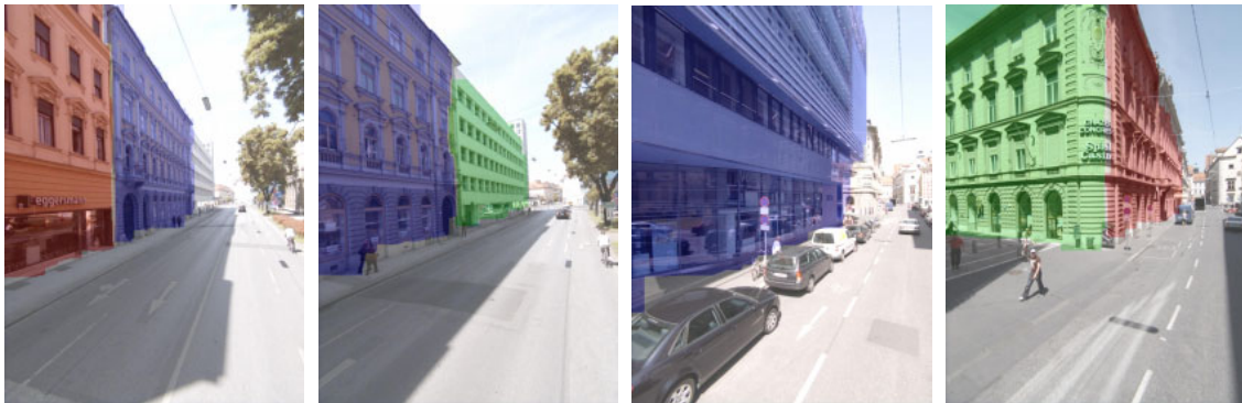
Separation and segmentation results for different facades in a multi-view scenario (large kernel setting). Even for facades under perspective distortion, the multi-view scenario provides robust results.
