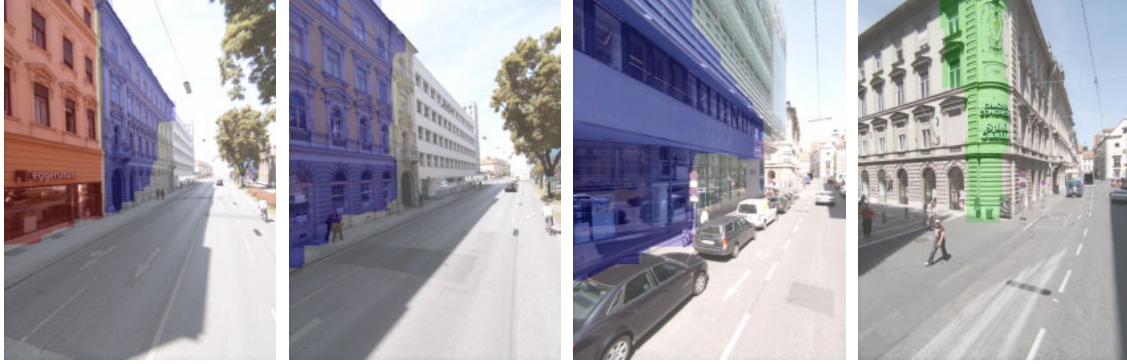
Figure 10. Separation and segmentation results for different facades in a single-view scenario (large kernel setting). While separate facades are found in general, the algorithm in the single-view scenario does not always provide complete façade segments and is not able to detect as many separate facades as in the multi-view scenario.
