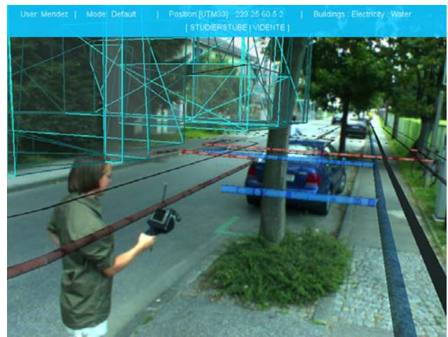
Figure 10: View through the AR display deployed outdoors. In the image a second AR user with a handheld AR display can be seen. On the left, wireframed building models are displayed to retain spatial context.
