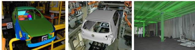
Figure 1: Applications of reconstructed models (from left to right): Occlusion problem in AR scenarios due to missing depth information of real environment (figures courtesy of Adam Opel GmbH); Collision detection and minimal distance calculation; Discrepancy check (figures courtesy of Volkswagen AG)
