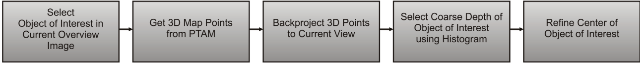
Figure 3. For selecting the area of interest (AOI), the inspector selects a rectangular region in the current view on the tablet computer. The depicted selection pipeline is then used to define the object’s center and size in 3D world coordinates.
