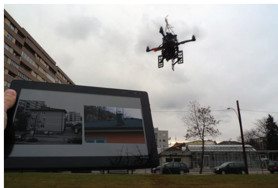
Figure 1. Our inspection system is capable of providing wide field-of-view low-resolution overview images (left) and high-resolution detail images with a narrow field of view (right) using a single industrial camera mounted on an MAV. The inspector can interact with the tablet computer to select an arbitrary object of interest.
