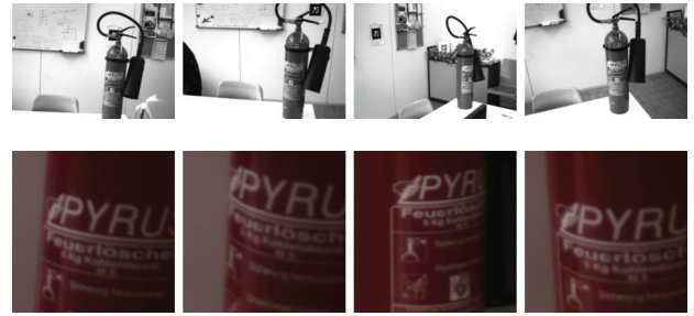
Figure 8. A series of large view point changes. In the top row the overview images are depicted, and in the lower row the tracked detail images. It can be seen that an inspection of one object from different view points is possible without reselecting the object of interest.
