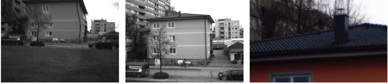
Figure 5. Comparison of image acquisition methods: (a) shows a full-resolution, full-frame image with considerable motion blur and rolling shutter effects. In contrast, our approach delivers (b) a binned full-frame overview image used for visual servoing and (c) a cropped full-resolution detail image used for inspection.
